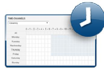
**Time Channel** Limit a group's use by setting a time channel. The group's keys are available when the time channel is active.
