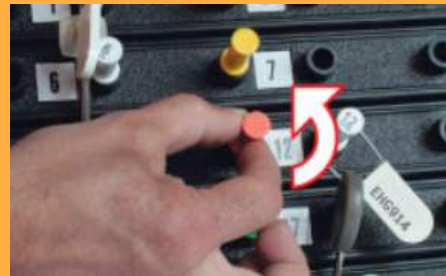
By turning the access peg the system is activated and the desired key is released
