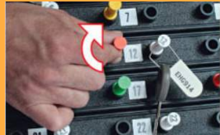
The colored access peg is inserted to remove the desired key from the system
