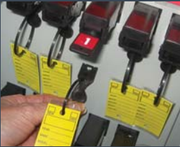
Returning the vehicle keys releases the Access Key
